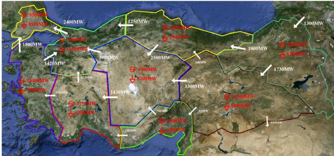
Figure A 2-8: Summer Peak Inter-Regional Projected Load Flows in 2017. (Source: TEİAŞ & TUBITAK, 2013 201 ).
