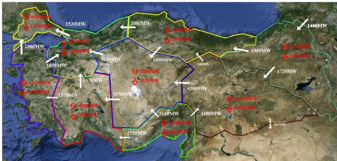
Figure A 2-9: Summer Peak Inter-Regional Projected Load Flows in 2022. (Source: TEİAŞ & TUBITAK, 2013 202 ).
